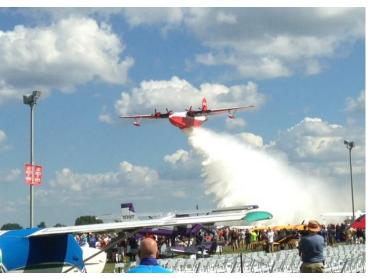
The Hawaii Mars, a flying boat water bomber, able to scoop and release 7,000 gallons of water performed a demo during the airshow on opening day.
