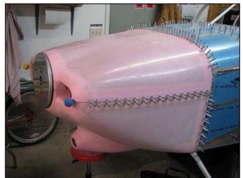
The piano hinges have yet to be riveted on. Van's suggests supplemental bonding of the hinge to the cowl.
