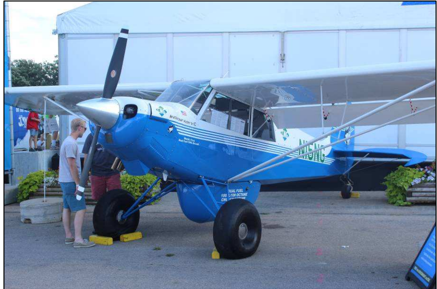
The Aviat Husky with a bulbous tank on the belly for compressed natural gas.
