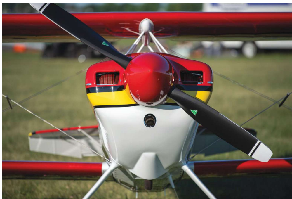
The MT constant speed prop helps keep the rpm down while putting 200 hp into the airstream.
