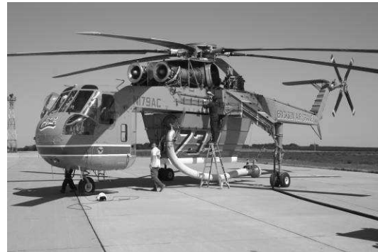
Erickson Air-Crane in its firefighting mode. The "hover snorkel" can refill the tank in 45 seconds!
