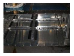
I masked off the area next to the rib with electrical tape. It made cleanup a little easier.
