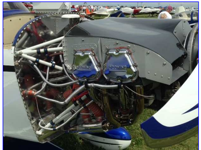
Lycoming IO-360 engine with a Whirlwind RV-74 propeller. 2600 RPM, 7500 FT, 100 ROP = 199 knots.
