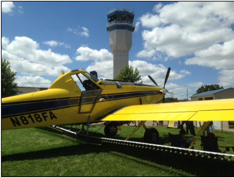
It's incredible how big these Ag planes are. This is an Air Tractor 802. Engine SHP: 1,295 @ 1,700 RPM. Wing Span: 59.2 ft. Hopper Capacity: 800 US gallons.
