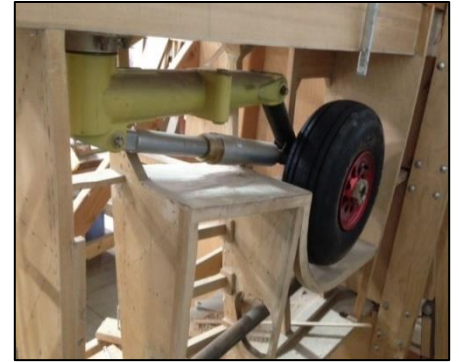
The Falco utilizes a retractable landing gear.
