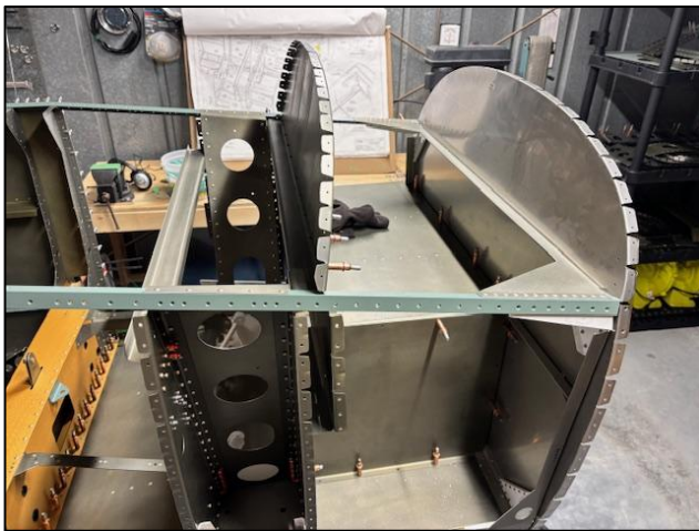
Main longeron riveted to the firewall/engine mounts.
