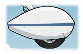
only going to put on one layer of glass on this side. All the sanding/grinding prep is done with very coarse sandpaper (60 to 80 grit). Any area that will be repaired must be sanded completely dull. Vacuum the repair area.
