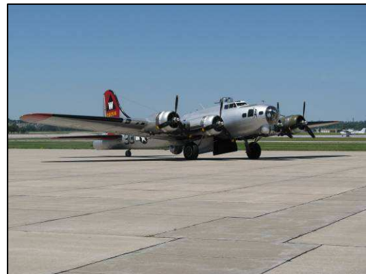
Each day began cranking each prop 9 blades to circulate the oil in the 1200 hp radial engines. This was definitely a 3 to 4 person job.
