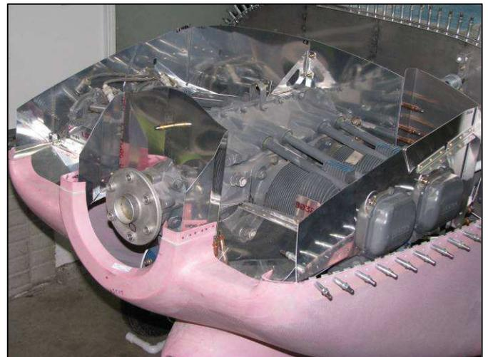
**I've been pleased with the engine baffle kit from Van's. Most everything is pre-cut with very little trimming to do.**
