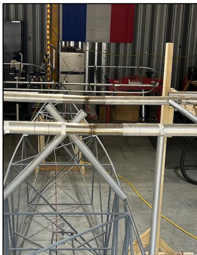
Top wing with stainless steel insert joining both sides. If the wing fails under load, it will not be here.
