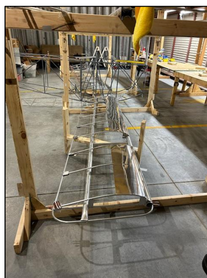
Lower right wing after spars, ribs, rib gussets for trailing edge and leading edge covering installed
