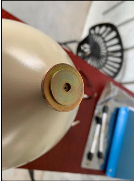
Once I had this marked, with the prop already on the plane, I clamped the spinner in place. I then took a ladder and with a pencil clamped to it, placed the point of the pencil right in front of my mark on the cone. If the spinner is in perfect alignment, the mark on the cone will remain in position through a full 360 degree rotation.
