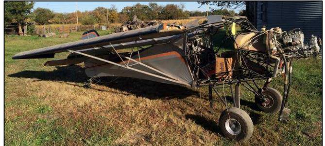
It was ground looped and bent the frame, which has been repaired but needs fabric stretched over it. The left wing is bent and damaged starting about 4 feet from the end, but the right wing is fine. Prop strike, but fiberglass propellers just broke off. Engine is a Rotax 582.
