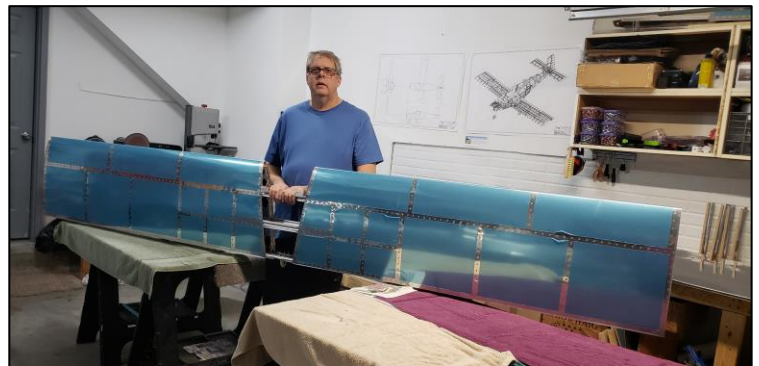
Bruce Holtmeier has completed the horizontal stabilizer on his RV-10.
