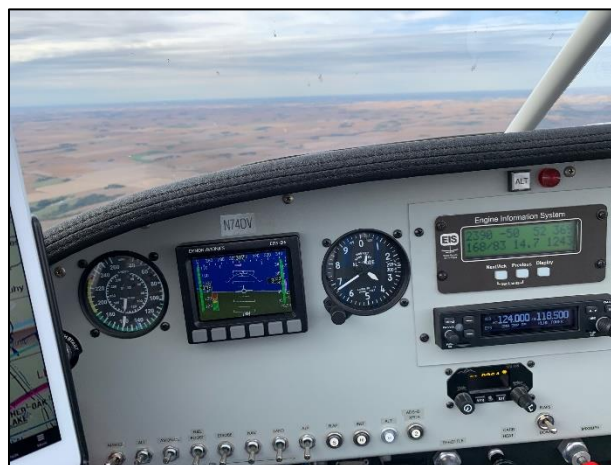
The big three, Engine Information System (GRT EIS 4000), Comm Radio (Garmin GTR 200) and Transponder (Sandia STX 165) have performed flawlessly.
