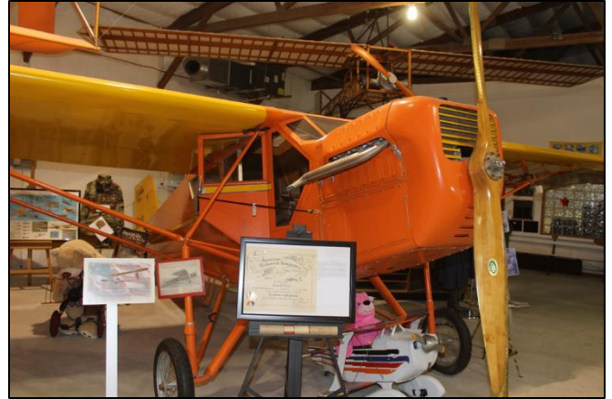
This rare Curtis Robin is the third built and the oldest surviving aircraft of its type. It used a surplus WW-1 OX-5 engine.
