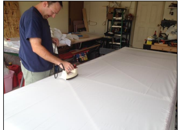
Derek Schroeder is making good progress on his Challenger 1. Here he is ironing the wrinkles out on his wing. The fabric he is using is Superflite 104.
